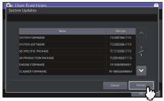
Connect your USB storage device in which the files for updating the system are stored to the USB port on the equipment, and press [OK].
