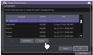
2 Connect your USB storage device in which the language pack is stored to the USB port on the equipment, and press [OK].
