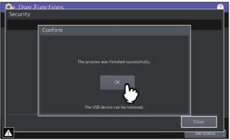
**Remove the USB storage device from the USB port on the equipment.**
